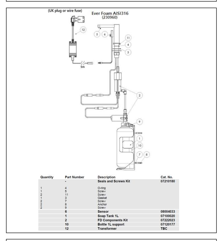
Note: In order to locate the relevant spare part, please check the corresponding parts and part mumber in the drawing. Minimum order quantity will be required.
